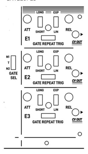
There are three identical linear-exponential evelope generators with Attack and Release time controls
