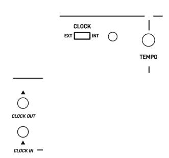
CLOCK pulses are generated internally at the rate set by the TEMPO control. With external clock the TEMPO control becomes a clock divider, ranging form 1 to 6. It is possible to sincronize a Clock24 signal or even a MIDI clock as long as the clock is the only signal appearing on the MIDI line.
